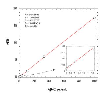
**Lower Limit of Quantification (LLOQ):** Triplicate measurements of serially diluted calibrator were read back on the calibration curve over 2 reagent lots across 3 instruments (13 runs total).
