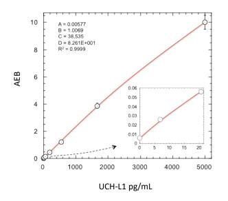
**Lower Limit of Quantification (LLOQ):** Triplicate measurements of serially diluted calibrator were read back on the calibration curve over 1 reagent lot on 1 instrument (5 runs total).
