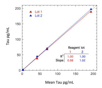
**Reproducibility across Lots:** 17 spiked and native serum tau samples (range 1.71-487 pg/mL, and 9 CSF samples (range 119-713 pg/mL) tested with 2 reagent lots on a single instrument in a single run.
