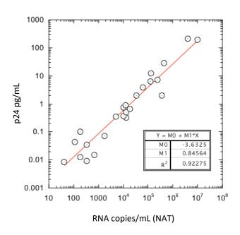
Lower Limit of Quantification (LLOQ): Triplicate measurements of serially diluted calibrator were read back on the calibration curve over 1 reagent lot across 2 instruments (3 runs total).
