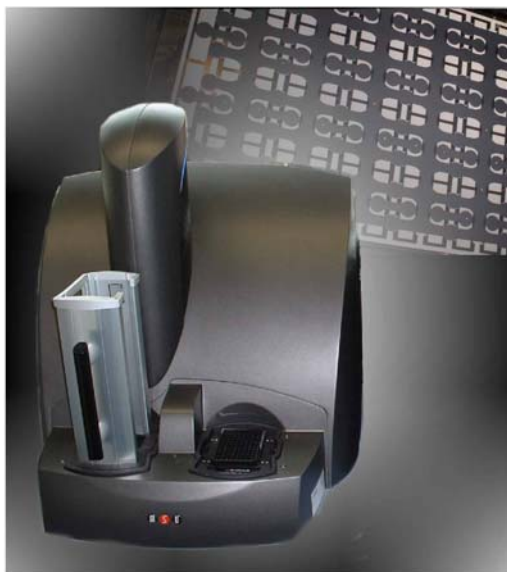
Figure 3A. Meso Scale Discovery (MSD ® ) ECL-detection system: an optimized combination of functional plate material and automated reader for high-throughput multiplex analysis.
